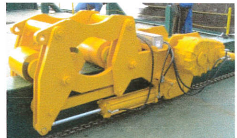
Conductor Handling Tool: for 36" and 48" pipe. Barge mounted. Utilized by Petrobras and Shell in Brazil.
