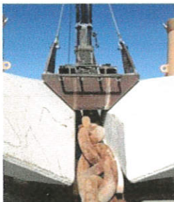
Chain Tensioning Mechanism: for BP pipeline anchoring
