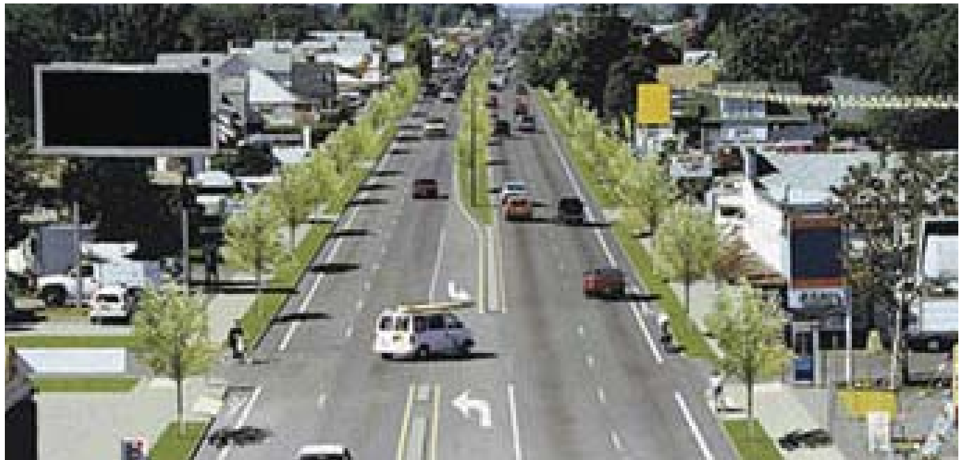
median and turn lane channelization example
